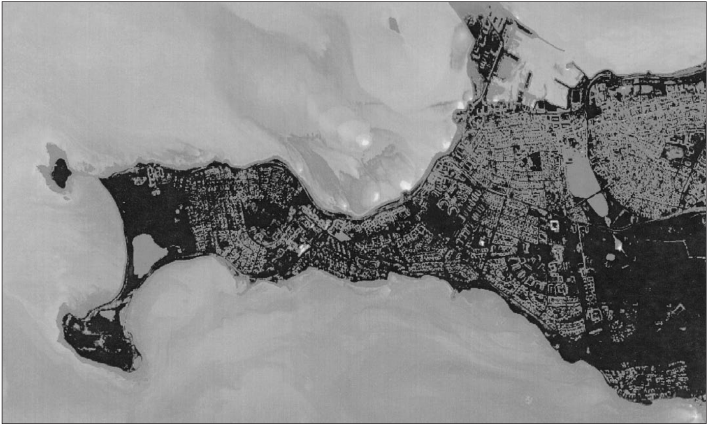
Remote sensing creates possibilities for work on planning and environmental matters. The figure shows the scale of surface temperature, light being hottest, dark coldest. Sewer discharge and the distribution of pollution are clearly visible.
