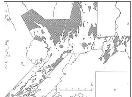
Dark areas define areas that fit badly for road building because of steep or uneven terrain.
