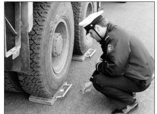
Loads have to be controlled because of the limited carrying capacity of roads.
