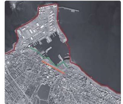
EFLA has defined three alternative sea walls to defend the Harbour and Kvos
